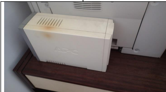
58. UPS APC - neispravan
